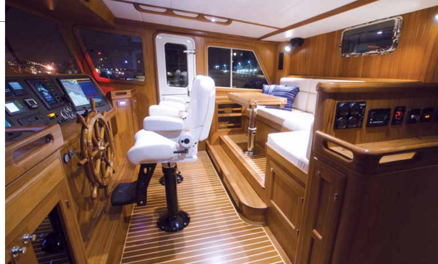
Ergonomics play a vital part in the pilothouse layout, which is well proportioned to include room for twin helm seats, plenty of walk-through room behind the seats to make it easy to access the Dutch-style doors on either side, and a comfortable raised bench seat behind with a drop-down table that converts into a double berth for the off-watch.
