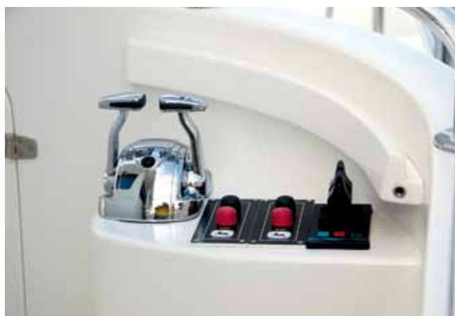
Left: The massive Portuguese bridge wrapping around the front of the Krogen 52 pilothouse features a hawse with cleats for easy fender positioning, a sturdy stainless steel grabrail, and storage lockers accessed from the back. Top right: Two well-spaced anchors on the bow are served by a Maxwell HWC 3500 windlass. Bottom right: Twin wing stations include throttle and shift binnacles, engine start and stop switches, and thruster controls.
