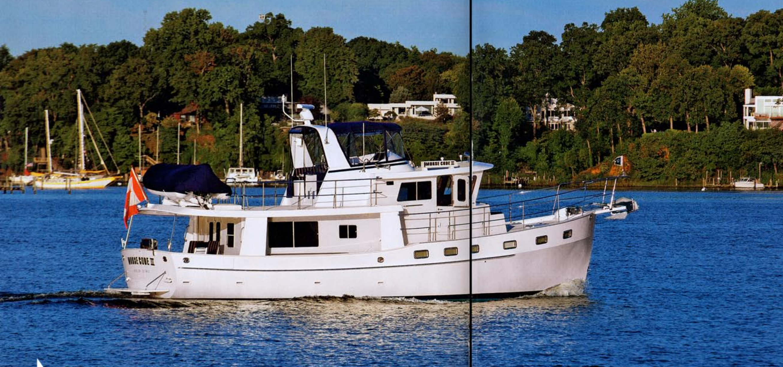
The shape of Kadey-Krogen's Pure Full Displacement hull is essentially the same for all models. A fine bow and wine-glass transom
