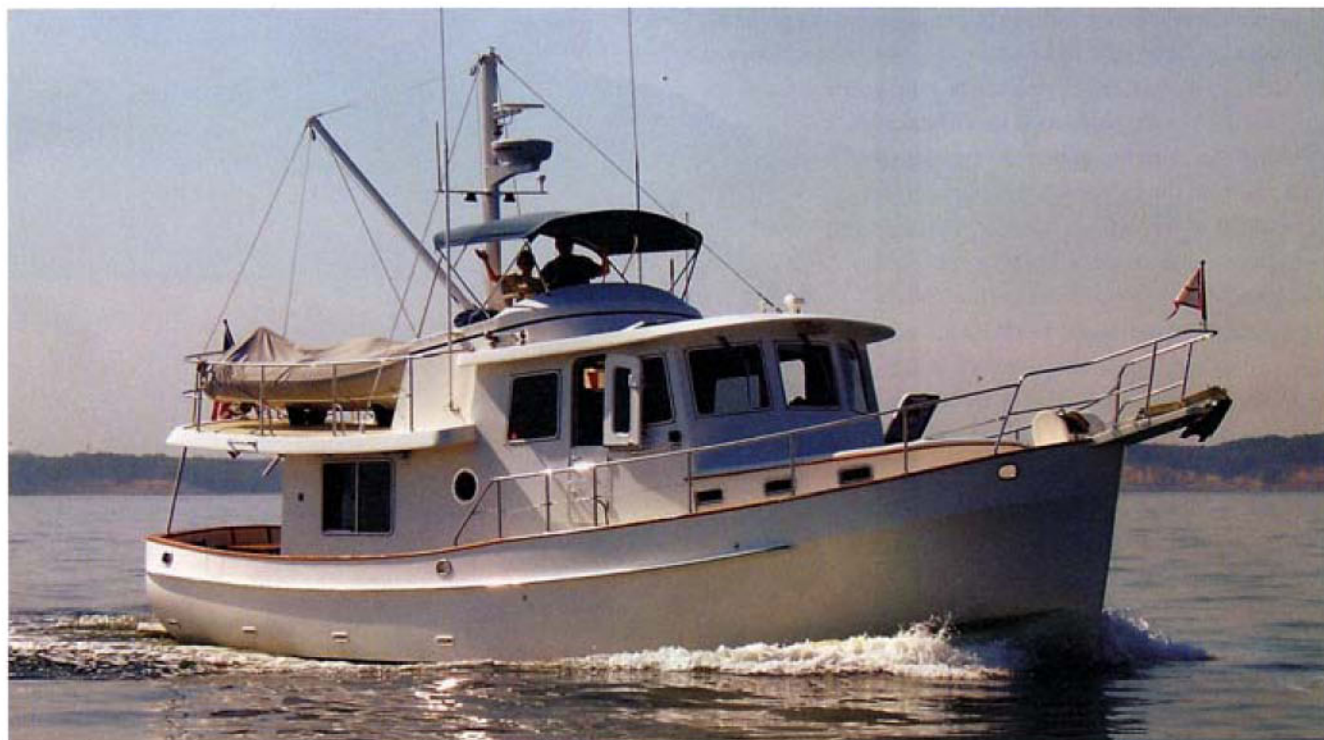
Sweet Time, a Kadey-Krogen 39, pushes a smooth wake from her sharp forefoot to her wineglass transom as she cruises close to hull speed.
