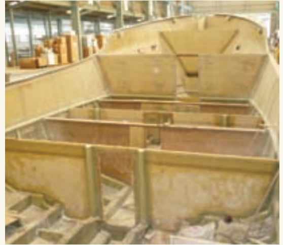
Bulkheads are tied into massive stringers.
