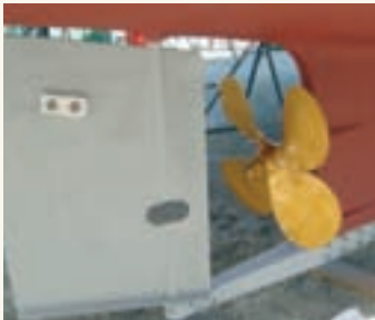
Stainless rudder with shoe
