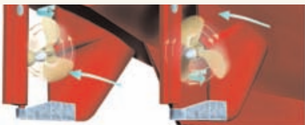
Counter faired keel imparts counter water rotation.
