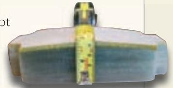
competition: an aramid reinforced hull. This aramid fiber is stronger than ballistic steel and is the same fiber used to give body armor its "bullet-proof" capability.
