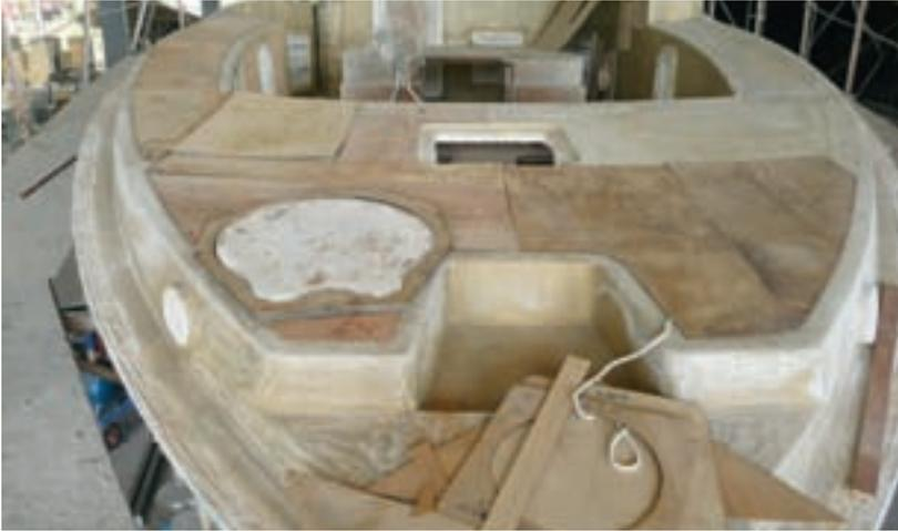
Structures are reinforced with fiberglass stiffeners.
